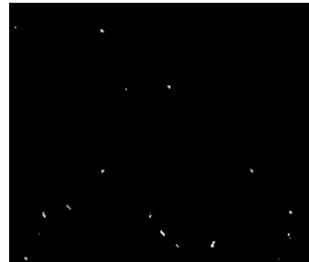
Diesel fuel at cloud point A few wax crystals appear instantaneously
